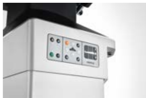
Override panel (Backup control panel)
